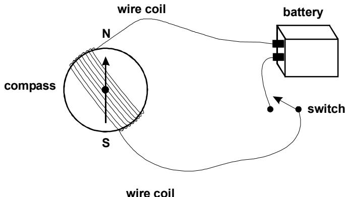
A student coils a wire around a compass to make the circuit shown above. The student observes that the needle of the compass is deflected from its north-south position whenever the switch in the circuit is kept closed. When the switch is kept open, the needle is not deflected from the north-south position. Which of the following best describes why this occurs?
